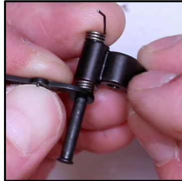
Step 18: Push the Pin almost all the way out to make room for the New Flat Trigger.
