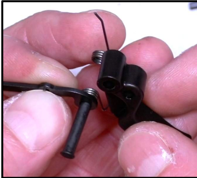
Step 18: Push the Pin almost all the way out to make room for the New Flat Trigger.
