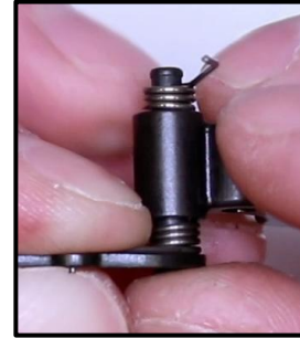
Step 20: Push the Long Leg of the Trigger Spring up behind the Barrel.
