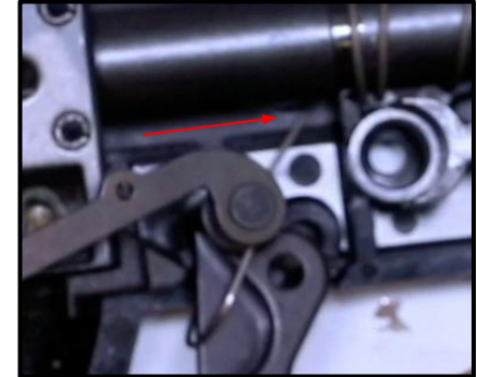
Step 20: Push the Long Leg of the Trigger Spring up behind the Barrel.
