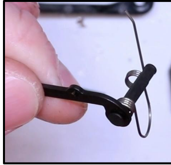
Step 18: Push the Pin almost all the way out to make room for the New Flat Trigger.
