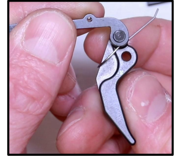
Step 20: Push the Long Leg of the Trigger Spring up behind the Barrel.
